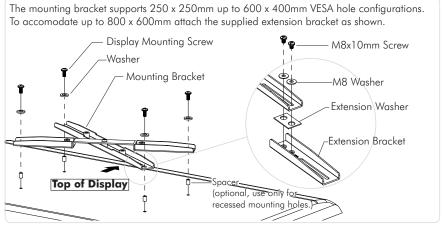
Step 6. Insert two M8x16 Screws
